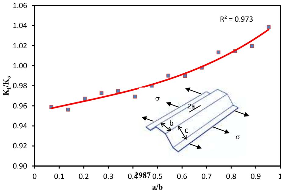
Figure (7) Effect of crack length on shape factor C
