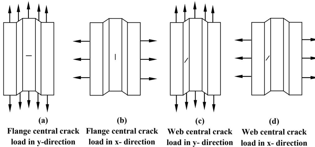
Figure (2) Crack location and load direction for each case
