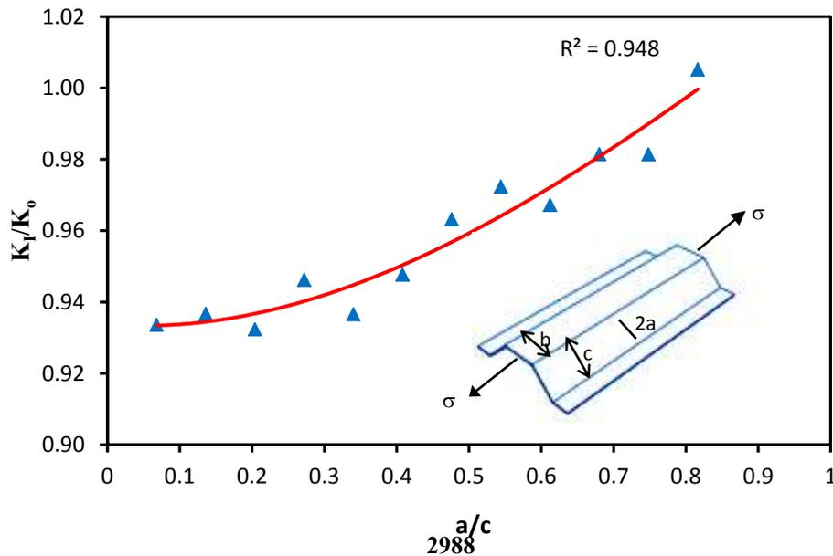
**Figure (9) Effect of crack length on shape factor C**
