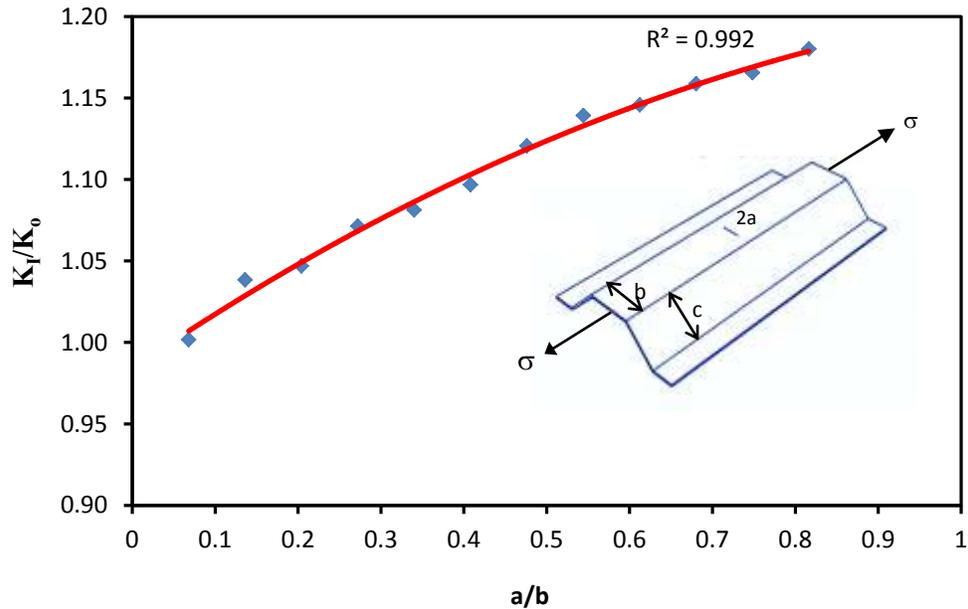
Figure. (4): Effect of crack length on shape factor C
