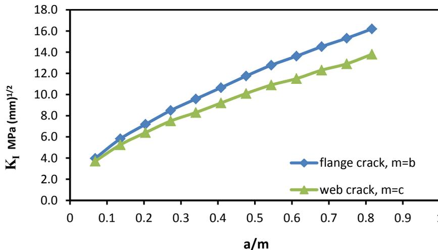
Figure (3) Effect of crack length on the stress intensity factor  $K_I$
