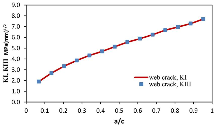
Figure (11) Effect of crack length on the stress intensity factors  $K_I$  and  $K_{III}$
