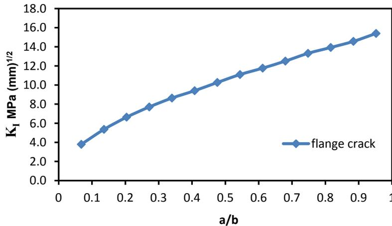
Figure(6) Effect of crack length on the stress intensity factor K<sub>I</sub>
