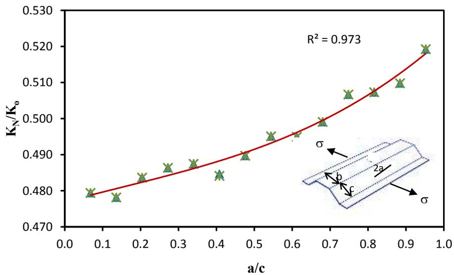
Figure (12) Effect of crack length on the shape factor
