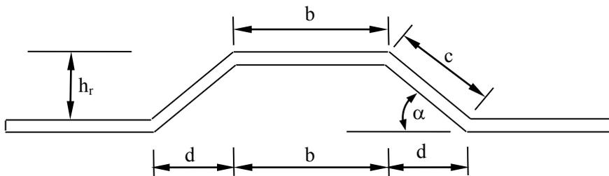
**Figure (1) Corrugated plate geometry [7]**
