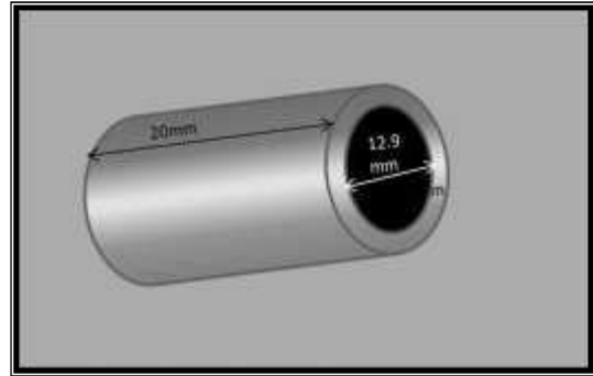
Figure (2) tensile specimen coupon dimensions centimeters
