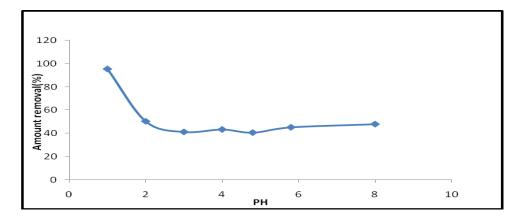
Figure(6) : Adsorption of (RB5) by (RHC) as a function of solution pH at initial concentration of 50 mg/l and adsorbent dosage of 1.5 g with 300µm particle size
