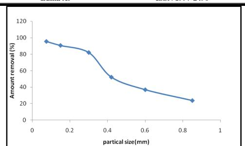
Figure(5) : Effect of particle size on adsorption capacity of (RB5) onto (RHC) at initial dye concentration of 50 mg/l and adsorbent dose of 1.5gm
