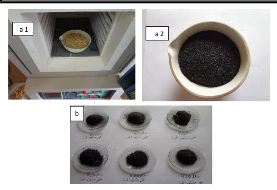
Figure(1): Iraqi rice husks used in this study. (a-1) The rice husks before burn (a-2) The rice husks after burn (b)-Granular rice husks carbon
