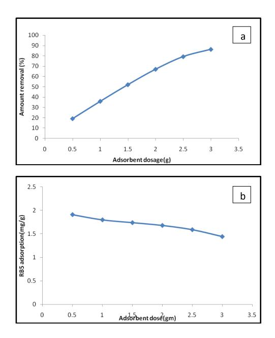
Figure (3) Effect of adsorbent dosage in the removal of RB5 by (RHC)
