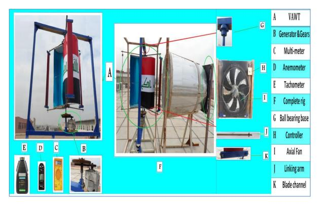
Figure (1): The designed small vertical axis wind turbine
