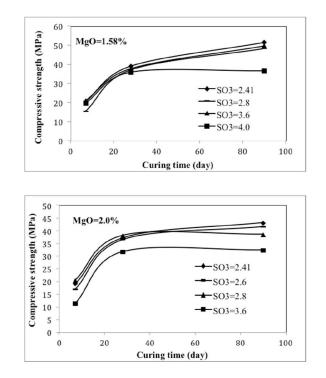
Figure 6 Compressive strength versus curing time with difference MgO and SO<sub>3</sub> contents in SRPC
