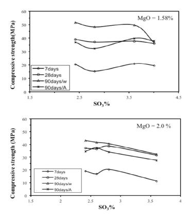
Figure 2 Compressive strength versus SO<sub>3</sub> content in SRPC with different MgO percentage
