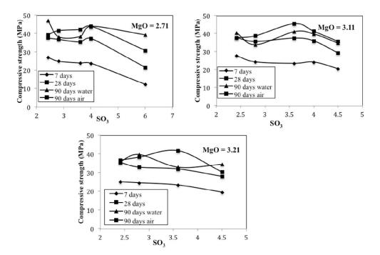
Figure 1 Compressive strength versus SO<sub>3</sub> content in OPC with different MgO percentage
