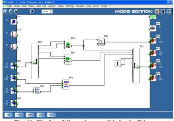
Fig. 10: The four I/O words accessible by the Ethernet communication module
