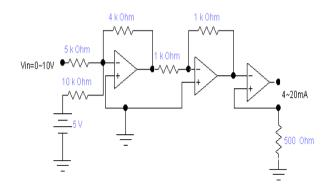
Fig. 12: Signal conditioner circuit that supplies the SCR with the required current signal
