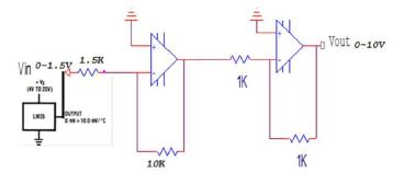
Figure 5: LM35 connection to signal conditioner Circuit
