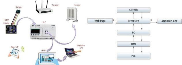
Figure 1: The overall architecture of the proposed system
