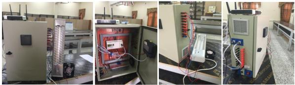
Fig. 17: The overall designed web- and Android-based PLC home temperature control system
