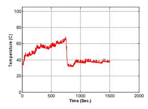
Fig.14: The real-time response of the PID temperature control system for two set points: 65°C and 40°C
