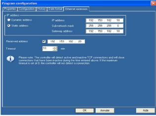
Fig.9 IP setting of Ethernet module
