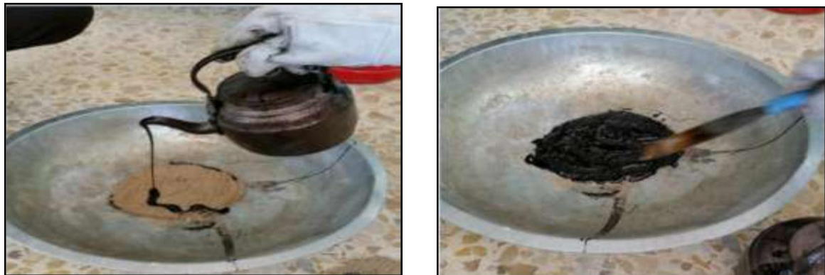
Figure 4: Bitumen coated Jute fiber sheet
