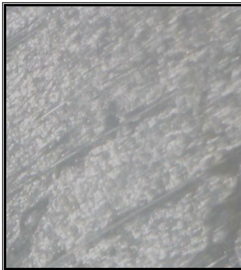
Figure (9) Buckling and fibrillation of fiber in local yielding
