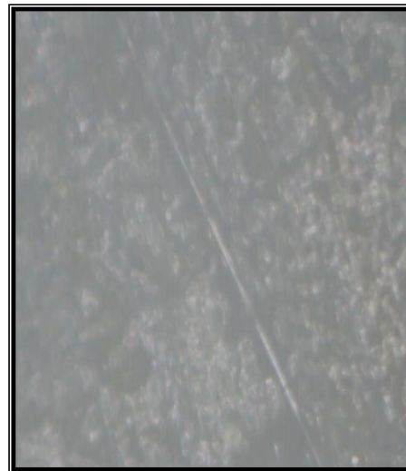
Figure (10) A single pull-out of E-glass-fiber from its matrix after deflection Loading
