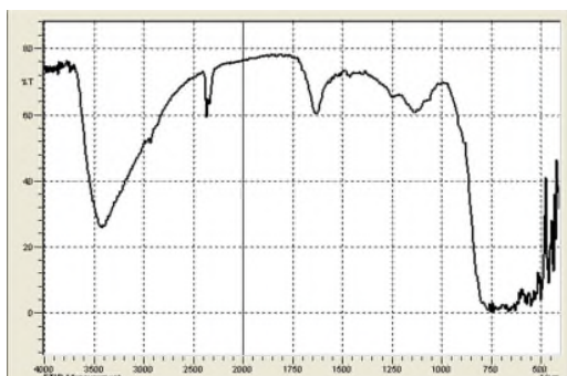
Figure (3) FT-IR spectra of pure TiO 2 nanoparticles prepared by sol gel method
