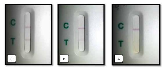
Figure 2: Illustration of the Positive and negative feed samples to residual Aflatoxins using total Aflatoxins rapid test strips. A: Positive for Aflatoxines 3ppb and more: Red T line is invisible, which means the content of Aflatoxins in sample is higher than 3ppb. B: Negative for Aflatoxines 0-3ppb, and C: Negative for Aflatoxines 0ppb: Red T line appears, which means there is no Aflatoxins residue in sample (C) or the content is lower than 3ppb (B).
