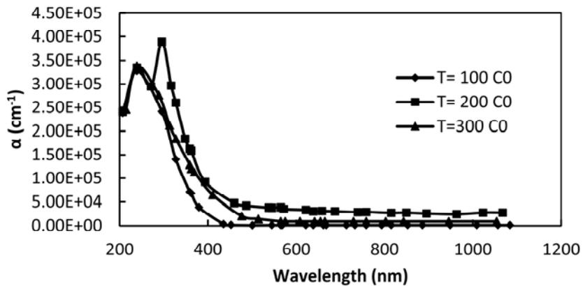
**Figure (3): absorption coefficient of CdO films annealed at different temperatures as a function of wavelength**
