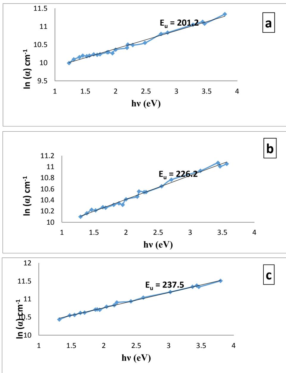
Figure(6): Variation of  $\ln(\alpha)$  Vs  $(h\nu)$  of CdO films annealed at different temperatures a)100 C°, b)200 C°, and c)300C°.
