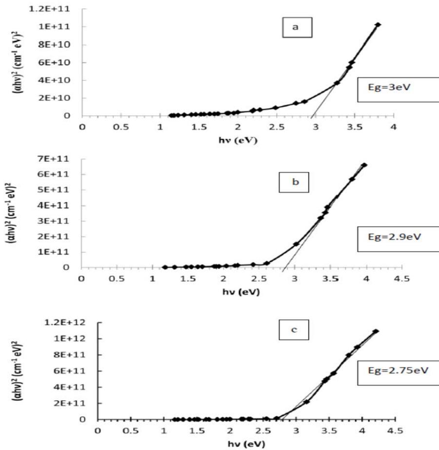
Figure(5): Variation of  $(\alpha hv)^2$  Vs  $(hv)$  of CdO films annealed at different temperatures a)100 C°, b)200 C°, and c)300C°.
