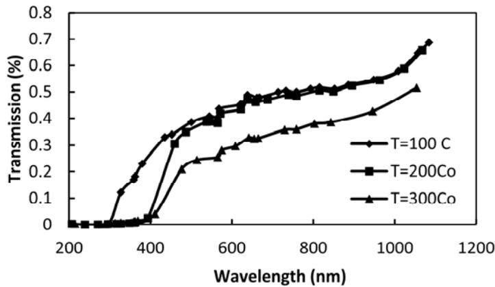
**Figure (2): Optical transmission of CdO films annealed at different temperatures as a function of wavelength.**
