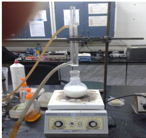
Figure (1) show reactor for synthesis of TiO 2 sol-gel
