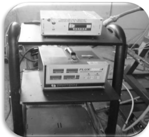
Fig. 2 b, Exhaust gases concentration measuring device type FLUX 2000
