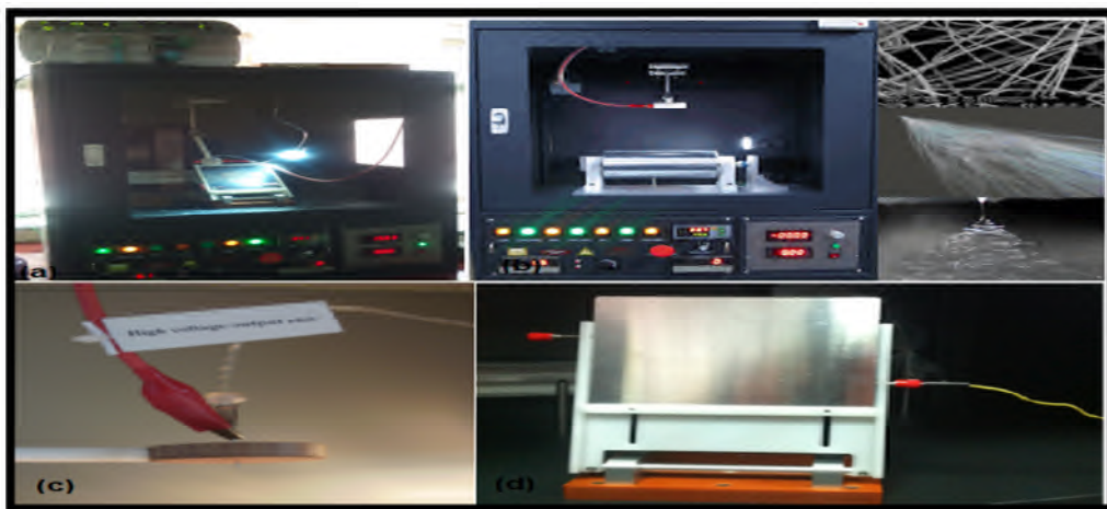
Figure(2): a-Nanobond Electrospinning system with rotation collector, b- with flat plate collector, c- needle connected to high voltage by upper electrode ,and d- flat aluminum plate collector connected to earthing lower electrode, with Taylor cone and spun image.
