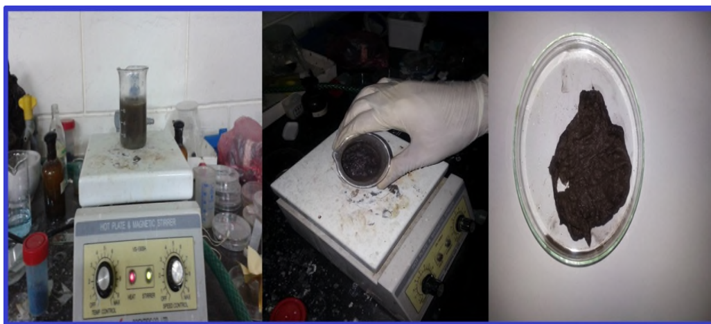
Figure (1) Preparation stages of cotton fiber coated by CuO thin film antibacterial
