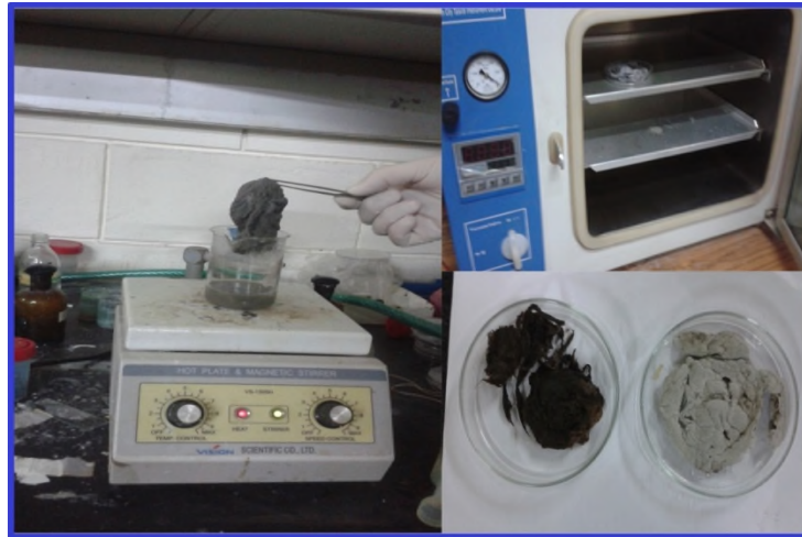
Figure (2) Preparation stages of cotton fiber coated by CuO and (CuO-TiO 2 - ZnO) thin films antibacterial after dried.
