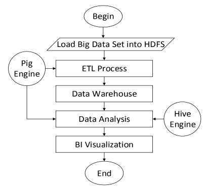
Figure (5), The Proposed System's Flowchart
