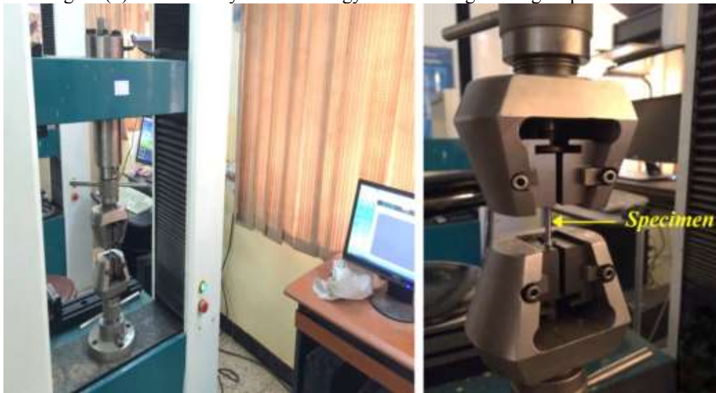
Figure(2) Tensile test machine WDW-200E.
