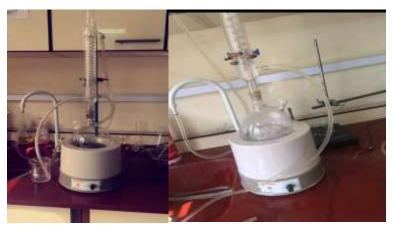
Figure (1): Reflux apparatus (Close system).
