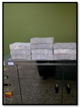
Figure (3) Concrete paving bricks specimens prepared in this investigation.
