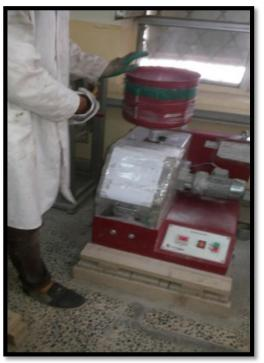
Figure (4) Abrasion resistance test for for concrete paving bricks.
