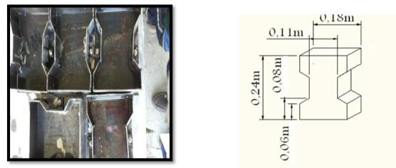
Figure (2) Molds and dimensions of concrete paving bricks.
