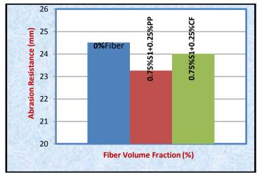
Figure (7) The Abrasion resistance of concrete paving bricks.
