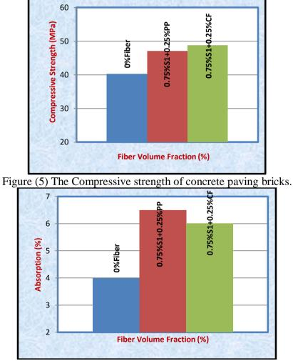
Figure (6) Absorption values of concrete paving bricks.
