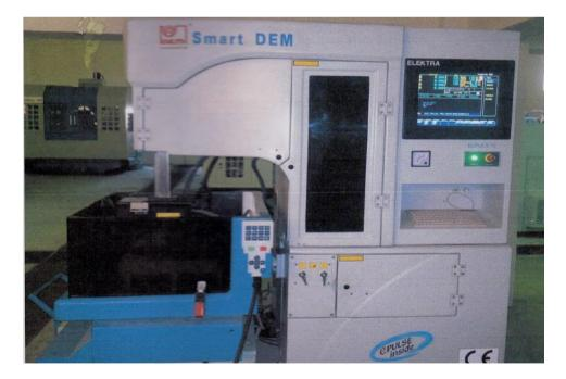
Figure (1) EL PULSE 5 Electra WEDM.
