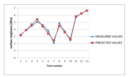
Figure (4) Relationship between measured and predicted Ra (coated wire).
