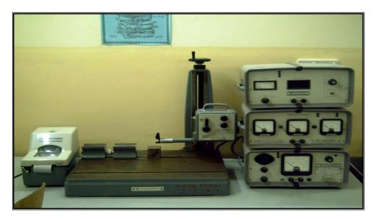
Figure (3) Roughness measuring apparatus.
