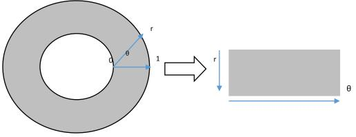
Figure (3). Polar to rectangular templates conversion.
