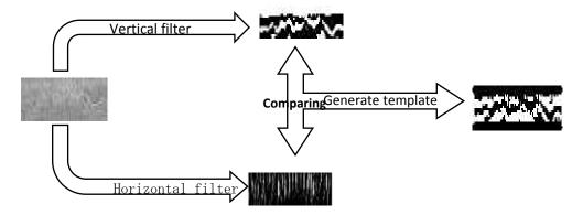
Figure(12). Ridge Energy Direction process for generating template
