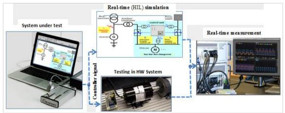
Figure (9) Demonstration of a hardware-in-the-loop (HIL) simulation
