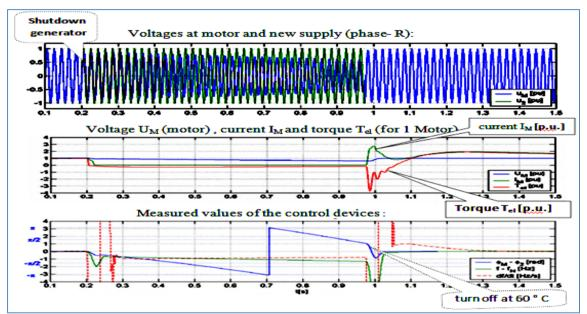
Figure (11): Timing a bus-bar/fast changeover
