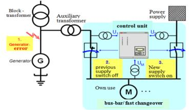
Figure (10) System configuration and control unit for abus-bar fast change-over
