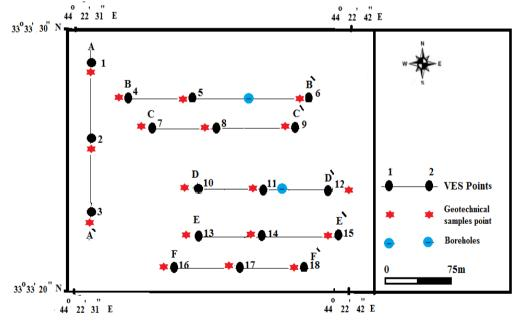
Figure (3) Data Acquisition Map of the Study Area Showing the Vertical Electrical Sounding Stations and the Geotechnical Sampling Points
