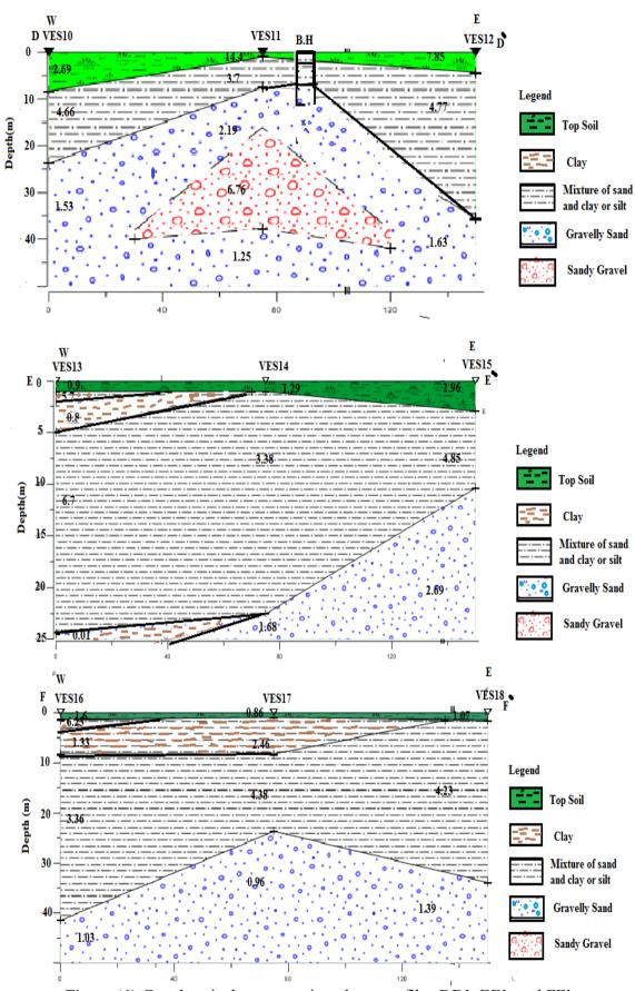
Figure (6) Geoelectrical cross section along profiles DD', EE', and FF'
