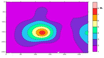
**Distance (m.)** Figure (8) Isopach Map of the Topsoil.
