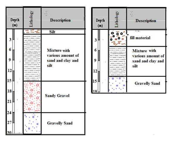
Figure (2) Soil section in B.H.1, B.H.2 in the study site after NCCL2000 (modified)
