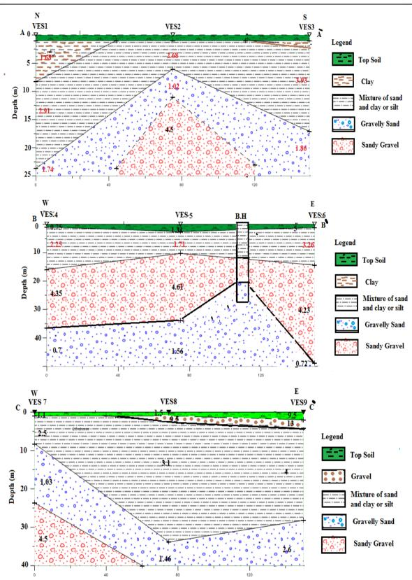
Figure (5) Geoelectrical cross section along profiles AA', BB', and CC'
