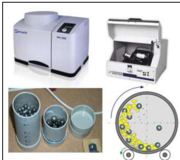
Figure 3a, general view of ball-mill equipment
