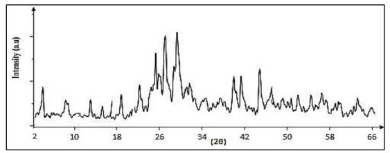
Fig. 2: XRD patterns, intensity versus 2 $\theta$  angle for the synthesized Nd:KTP structure doped by 10% of Nd in weight.
