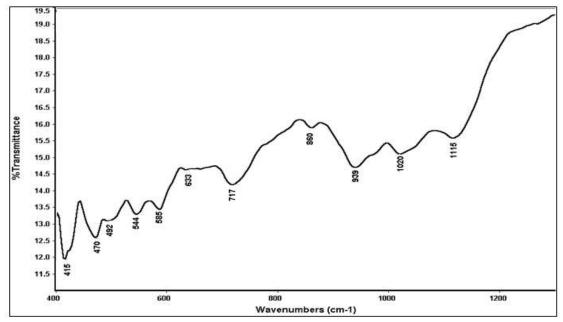
Fig. 3: FT-IR transmission spectrum of Nd:KTP nanocrystalline (10% Nd doping)
