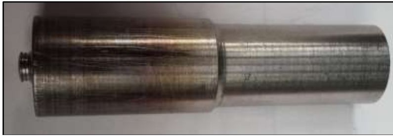
Figure(2): Threaded cylindrical pin tool used in this study.
