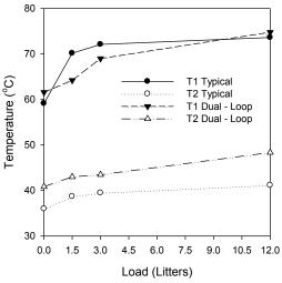
Figure (5): Variation the Inlet and Outlet Temperature of the Condenser with Load
