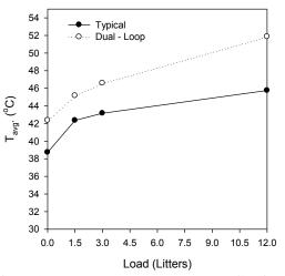
Figure (6): Variation of the Average Temperature at the Surface of the Condenser with Load
