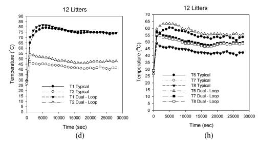
Figure (4): (a, b, c and d) the variation of temperature with time for inle and outlet of the condenser and (e, f, g and h) the Variation of the Average Temperature at the Surface of the Condenser (T6,T7 and T8) with all loads
