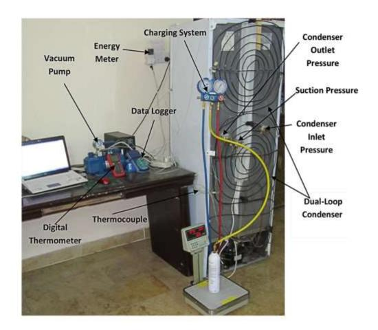
Figure (2) Experimental Setup of the Test Unit and Apparatus
