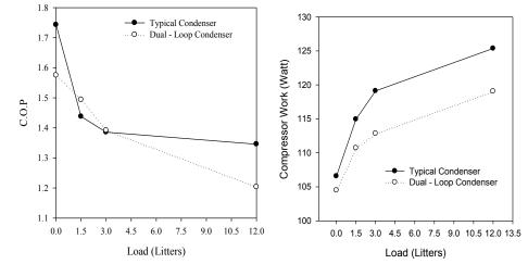
Figure (8): Variation the Compressor Work and the coefficient of performance with all Load
