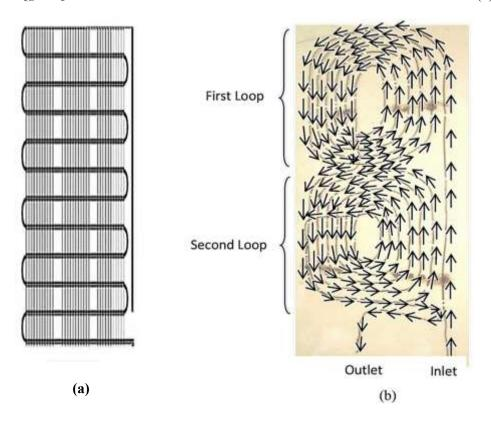
Figure (1): (a) Schematic of a wire-on-tube condenser and (b) dual-loop condenser
