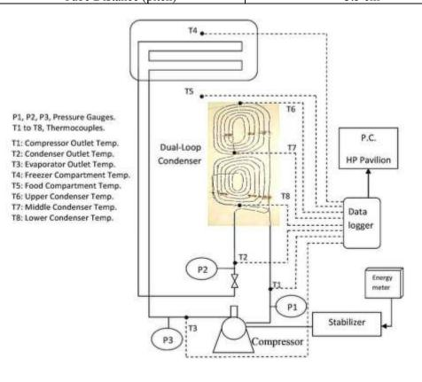
Figure (3)Schematic Diagram of the Test Unit and Apparatus
