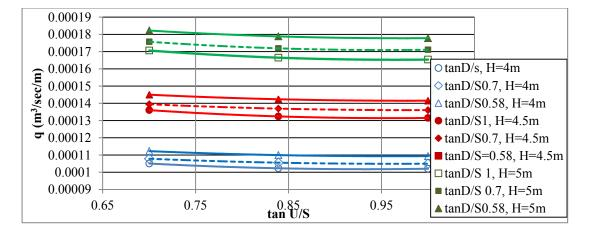
Figure.9. Relationship between (tan U/S) and (q) of triangular lining channel, Fb=0.5m, k canal 10-6 m/sec, k soil 0.0015m/sec.
