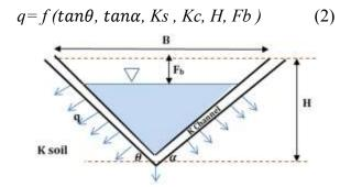
Figure. 3. The general section of triangular open channel with lining
