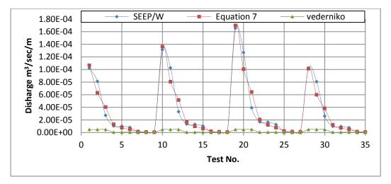
Figure. 16. Comparison between the calculated discharge for thirty tests with different method.
