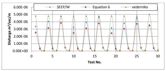
Figure. 17. Comparison between the calculated discharge for thirty five tests with different method.
