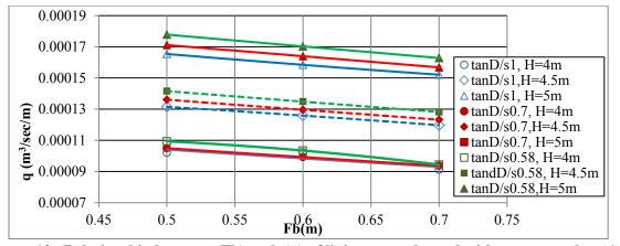
Figure.10. Relationship between (Fb) and (q) of lining open channel with upstream slope 1:1, k soil 0.0015m/sec, k canal 10-6m/sec.
