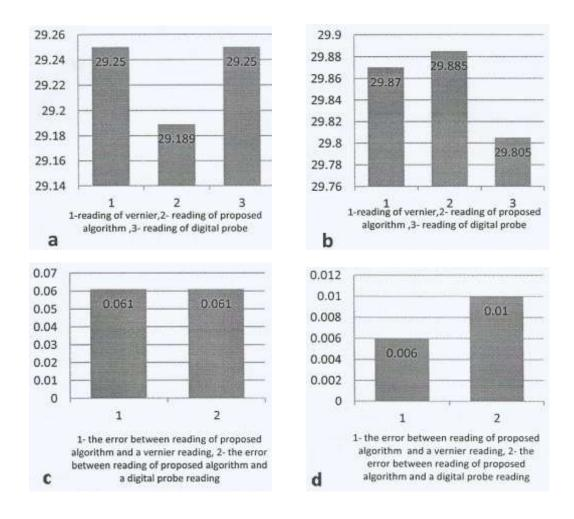
Figure(18) (a,c) comparison of digital vernier, scanning program and digital probe reading, (b,d) comparison the eroor of dimension for cylindrical shape
