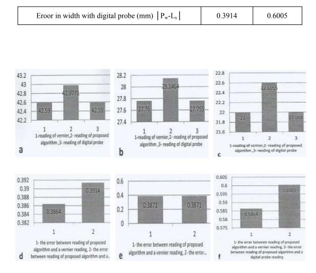
Figure(15) (a,b,c) comparison of digital vernier, scanning program and digital probe reading, (d,e,f) comparison the eroor of dimension for triangular shape
