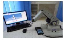
Figure (2) 5 DOF Lab-Volt R5150 Robot manipulator systems
