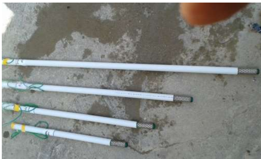
Plate (2) Watermark soil sensor inside PVC pipes and before installation.
