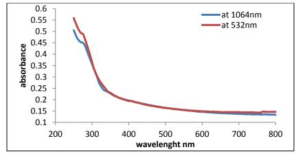
Figure(3) absoraption spectrumforTio2 NPsprepared by PLAL at two wavelength (1064nm ,532nm).
