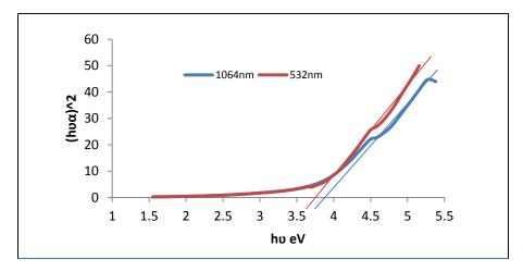
Figure(4) vairation  $(\alpha h v)^2$  with photon energy (hv) for TiO2 NPs
