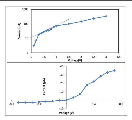
Figure (6):(a)the semi-log *I-V*characteristics plot(b)I-V dark characteristics of TiO2/Si heterjunction.
