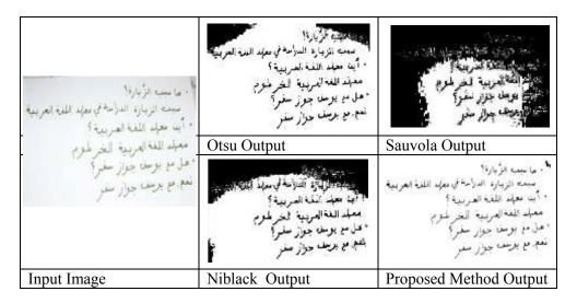
Figure (5) Comparative outputs of various thresholding methods and the proposed method
