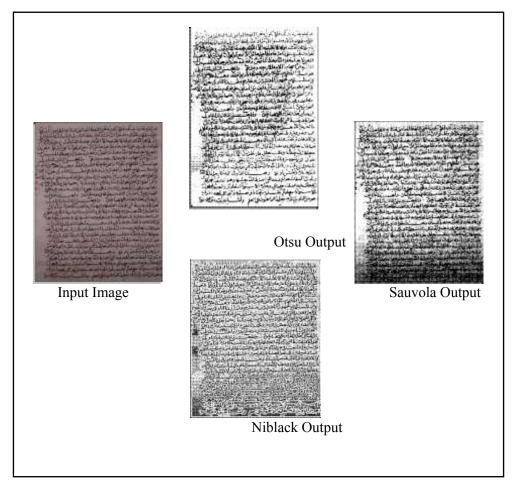
Figure(1)Images results of various thresholding methods
