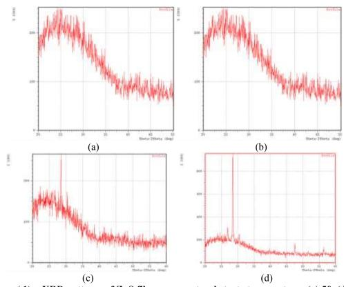
Figure (1): XRD patterns of ZnS films grown at substrate temperatures (a) 50, (b) 100 (c) 150 and (d) 200C<sup>o</sup>.
