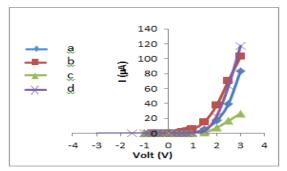
Figure (5): I-V characteristics for ZnS heterojunction prepared at various substrate temperatures (a) 50, (b) 100, (c) 150 (d) 200C°
