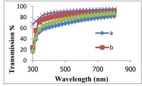
Figure(3): Transmission spectra of ZnS films on glass substrates with substrate temperature (a) 50 C°, (b)100 C°, (c)150 C°, (d) 200 C°.
