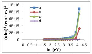
Figure (4) : Optical energy band gap for ZnS films at different substrate temperature of (a) 50 °C, (b) 100 °C, (c) 150 °C, (d) 200 °C.
