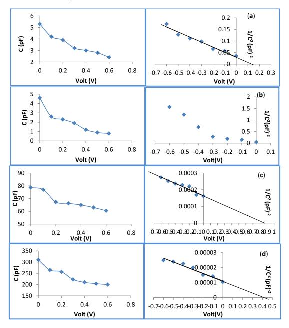
Figure(7): The variation of 1/C<sup>2</sup> versus reverse bias voltage for ZnS/Si heterojunction at different treatment temperatures (a) 50 C<sup>o</sup> (b) 100C<sup>o</sup> (c) 150C<sup>o</sup> (d) 200 C<sup>o</sup>
