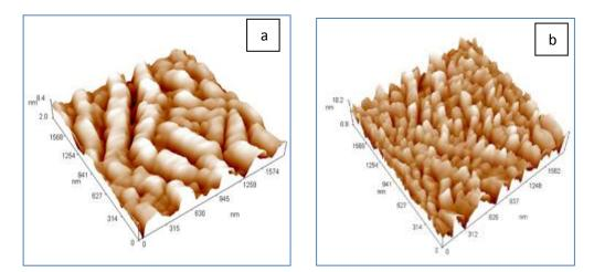
Figure (2): AFM images of ZnS films deposited on glass substrate at substrate temperatures (a) 50 and (b)150 C°.
