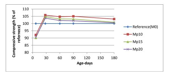
Figure (6): Compressive strength of HSC containing pumice as a percentage of reference specimens.
