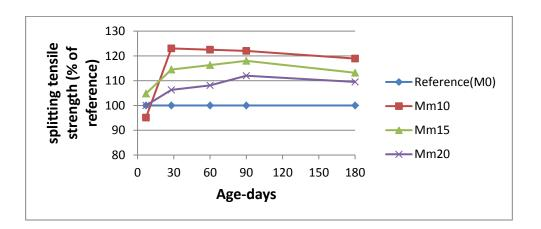
Figure (10): Splitting tensile strength of HSC containing MK as a percentage of reference specimens.
