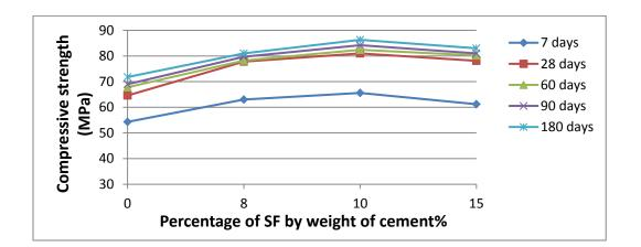
Figure (1): Effect of silica fume content(%) on compressive strength.
