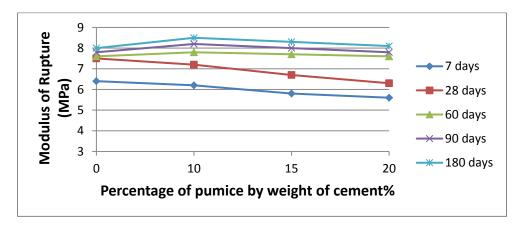
Figure (17): Effect of pumice content(%) on modulus of rupture.
