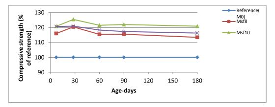
Figure (2): Compressive strength of HSC containing SF as a percentage of reference specimens.
