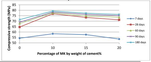
Figure (3): Effect of metakaolin content(%) on compressive strength.
