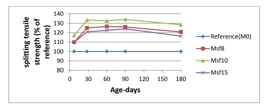
Figure (8): Splitting tensile strength of HSC containing SF as a percentage of reference specimens.
