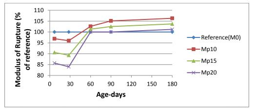
Figure (18): Modulus of rupture of HSC containing pumice as a percentage of reference specimens
