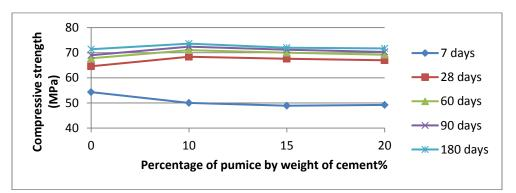
Figure (5): Effect of pumice content(%) on compressive strength.
