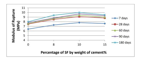
Figure (13): Effect of Silica fume content(%) on modulus of rupture.
