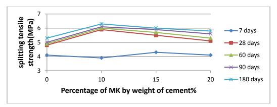
Figure(9): Effect of metakaolin content(%) on splitting tensile strength.
