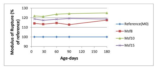
Figure(14):Modulus of rupture of HSC containing SF as a percentage of reference specimens.
