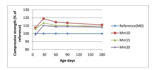
Figure (4): Compressive strength of HSC containing MK as a percentage of reference specimens.
