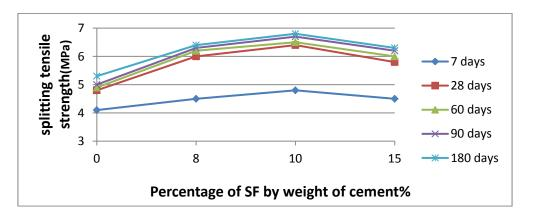
Figure(7): Effect of silica fume content(%) on splitting tensile strength.
