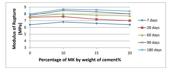
Figure (15): Effect of metakaolin content(%) on modulus of rupture.
