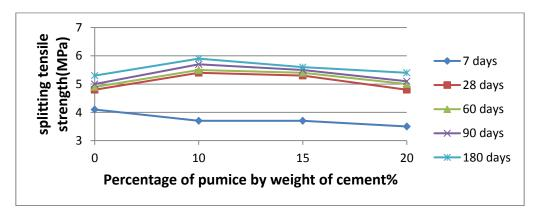
Figure (11): Effect of pumice content(%) on splitting tensile strength.
