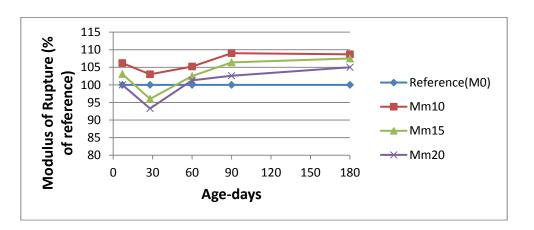
Figure (16): Modulus of rupture of HSC containing MK as a percentage of reference specimens.
