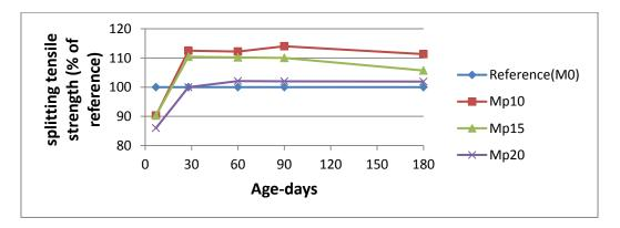
Figure (12): Splitting tensile strength of HSC containing pumice as a percentage of reference
