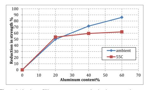
Figure 6 Aluminum filling content versus reduction in compressive strength
