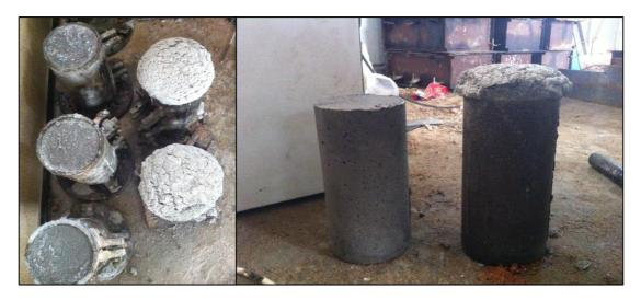
Figure 4 Swelling of specimens after short period of mixing and casting
