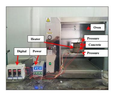
Figure 2 Thermal conductivity test
