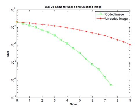
Figure (3): BER versus E<sub>b</sub>/N<sub>o</sub> for coded and Un-coded image
