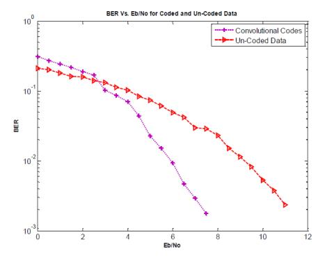
Figure (2): BER (bit error rate) versus E<sub>b</sub>/N<sub>o</sub> for Un-coded and coded data
