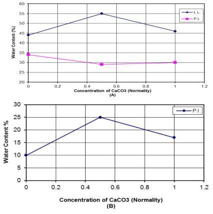
Fig. (2)Effect of Calcium Carbonate on Atterberg Limits
