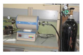
Fig. 6 Vacuum tube furnace.
