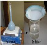
Fig. 2 The photographs of the (a) ZrO<sub>2</sub>-Cu coating powder succeeded on stirrer plate and filter,(b) ZrO<sub>2</sub>-Cu coating powder failure on stirrer plate and filter.
