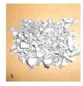
Fig. 3 The photographs of the (a) ZrO<sub>2</sub>-Cu coating powder succeeded after extraction from filter and milling ,sieved it below  $63\mu m$  (b) ZrO<sub>2</sub>-Cu coating powder failed.
