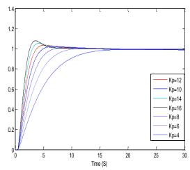
Fig. 7 step response for FOPDT for different values of Kp with FOPI controller.
