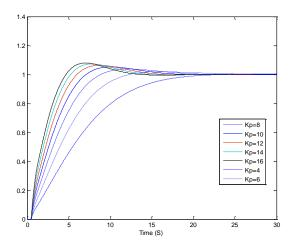
Fig. 8 step response for SOPDT for different values of Kp with IOPID controller.
