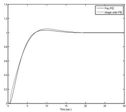
Fig. 3 step response for SOPDT.
