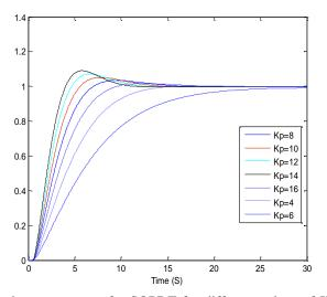
Fig. 9 step response for SOPDT for different values of Kp with FOPI controller.
