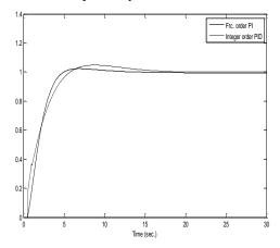
Fig. 2 step response for FOPDT.
