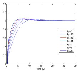
Fig. 6 step response for FOPDT for different values of Kp with IOPID controller.
