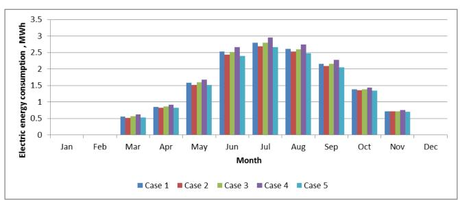
Fig. 8 Monthly space cool- electric energy consumption for different types of roof building material.
