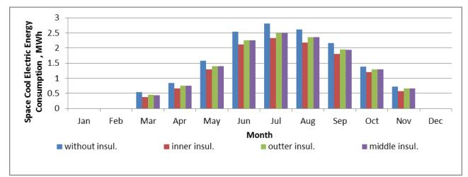
Fig. 12 Monthly space cool - electric energy consumption for different roof insulation position.
