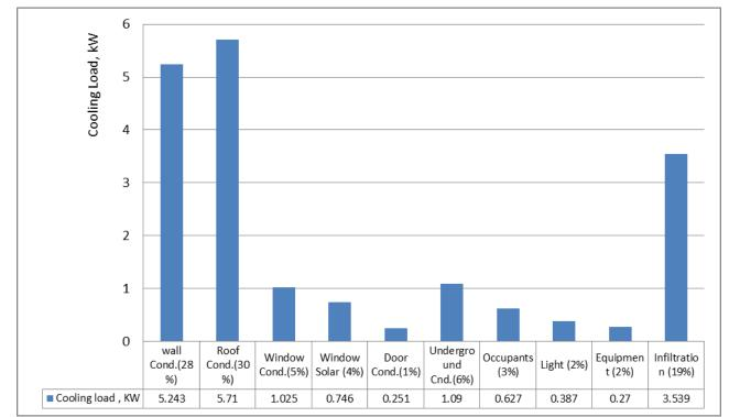
Fig. 3 Building peak cooling load components (Jul28th at 9PM) for the Base House.
