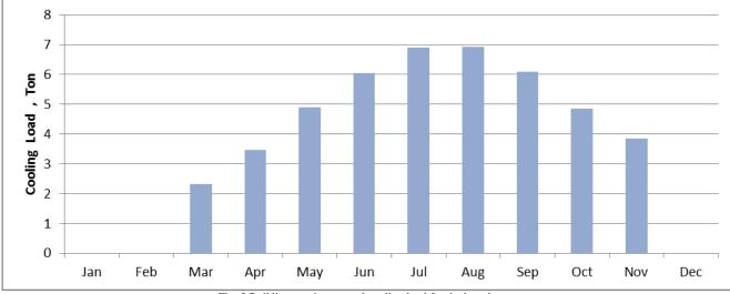
Fig. 5 Building maximum total cooling load for the base house.
