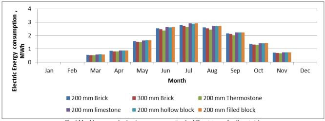
Fig. 6 Monthly space cool - electric energy consumption for different types of walls material.
