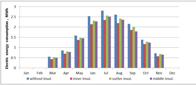
Fig. 10 Monthly space cool - energy consumption for different wall insulation position.
