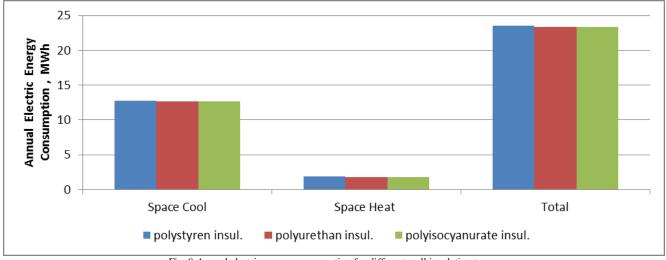
Fig. 9 Annual electric energy consumption for different wall insulation types.
