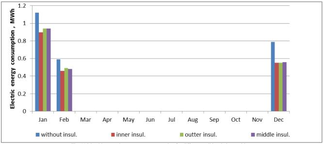
Fig. 11 Monthly space heat - energy consumption for different wall insulation position.
