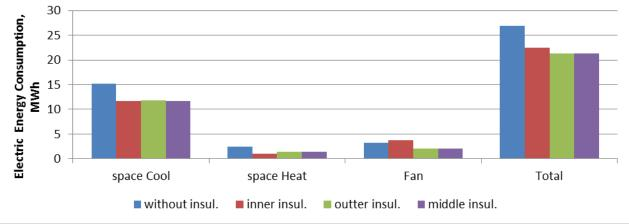
Fig. 13 Monthly space heat - electric energy consumption for different roof insulation
