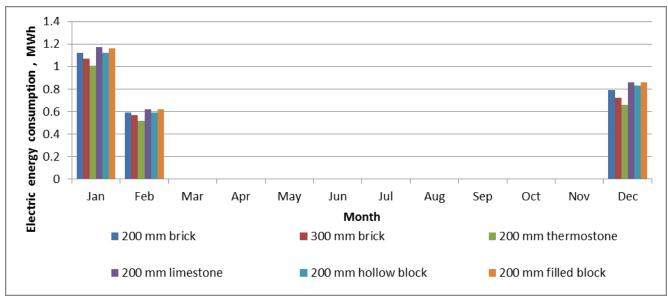
Fig. 7 Monthly space heat - electric energy consumption for different wall building material
