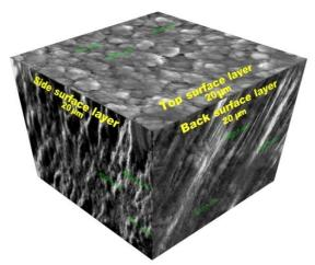
Fig. 9 Cubic body of SEM for 5083 roll wheel side ribbon, transverse side, and airside ribbon produced by RSP through OD of 2.5 mm, G of 2 mm and MT of 850 °C.
