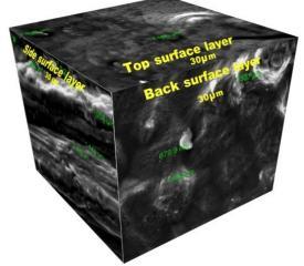
Fig. 4 Cubic body of SEM for 5052 roll wheel side ribbon, transverse side, and airside ribbon produced by RSP with OD of 2.5 mm and G of 2.5 mm at MT of 1000 °C.
