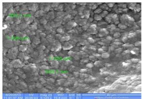
Fig. 8 SEM for 5083 ribbon produced by RSP through OD of 2.5 mm, G of 2 mm and MT of 850 °C.
