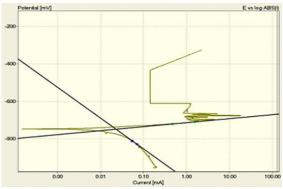
Fig. 11 CorrosionTafel plot for alloy type 5052 as received
