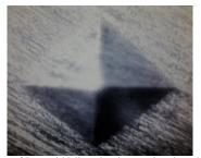
Fig. 10 Shape of Pyramid Micro-hardness printed on the specimen
