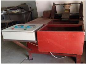
Fig. 1 Single roll melt spinning machine
