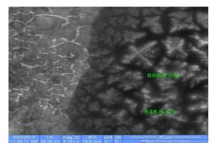
Fig. 7 SEM for 5083 ribbon produced by RSP through OD of 2.5 mm, G of 5 mm and MT of 850 °C.
