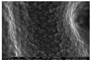
Fig. 6 SEM for ribbons type 5083 produced by RSP through OD of 2.5 mm, G of 2 mm and MT of 850 °C.
