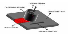
Fig.1 Schematic of friction stir processing (FSP) [5]
