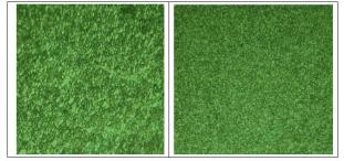
Nuggetzone for FSW at 1300rpm,60m Nuggetzone for FSP at 1300rpm,60mm/min Fig.14 the microstructure of nugget zone in FSW and FSP
