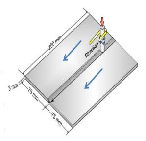
Fig.5 FSP process for 6061 – T6 plates FSW & FSP is done following the conditions that are shown in Table 4.
