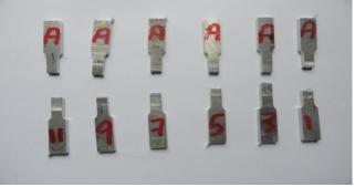
Fig.11 Tensile Test Specimen after testing
