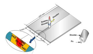
Fig.2 6061-T6 AA plates dimensions and Schematic of friction stir welding (FSW)
