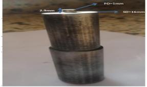
Fig.4 Tool for FSW and FSP
