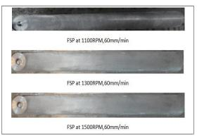
Fig.10 The appearance of upper surface of welding beads of 6061-T6 AA plates produced by FSP.
