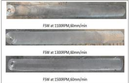
Fig.9 The appearance of upper surface of welding beads of 6061-T6 AA plates produced by FSW.
