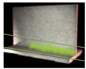
Fig. 4 Two colored parallel lines indicate the recommended arc length
