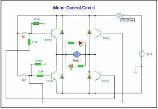
Fig. 5 motor control circuit
