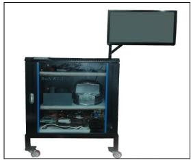
Fig.1Virtual Welding Training Machine (BasVW 1.1)
