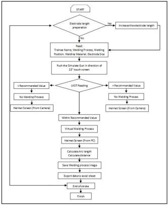
Fig. 6 Overall flowchart of electrode consumption simulation
