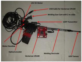
Fig. 3 welding electrode simulator
