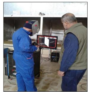
Fig. 2 Training one the virtual welding training machine (BasVW 1.1)
