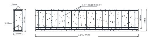
Fig. (1): Details of rectangular section (all dimensions in mm)
