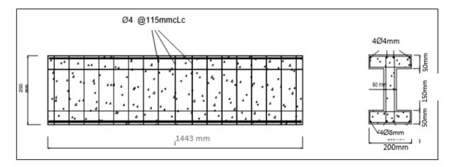
Fig. (3): Details of I-section (all dimensions in mm).
