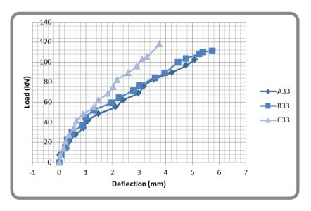
Fig. (11): Load -deflection curve for SCC I-section beam specimens with stirrups
