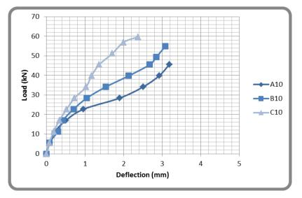
Fig. (6): Load -deflection curve for SCC Rectangular beam specimens without stirrups
