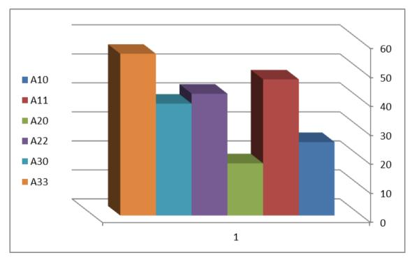
Fig. (14): Effect of absence of stirrups on the the ultimate shear strength at compressive strength  $(f_c)$  =29.36 MPa.
