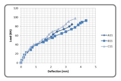
Fig. (7): Load –deflection curve for SCC Rectangular beam specimens with stirrups
