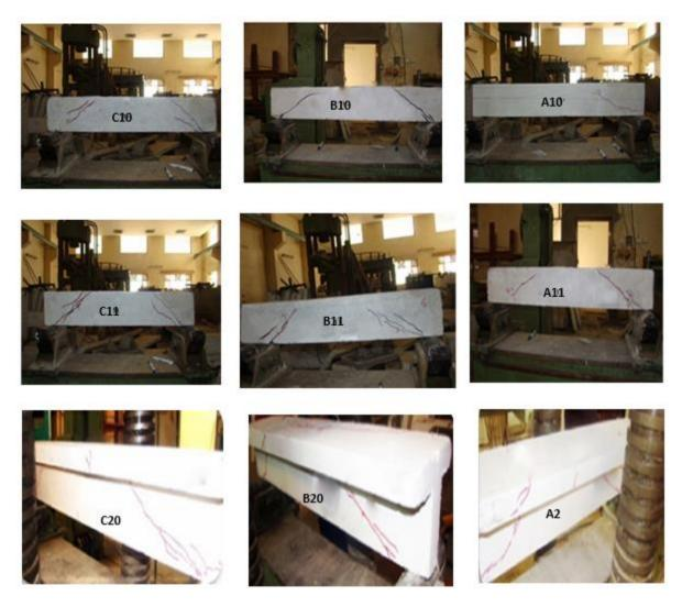
Fig (17): Crack pattern of the tested SCC beam specimens
