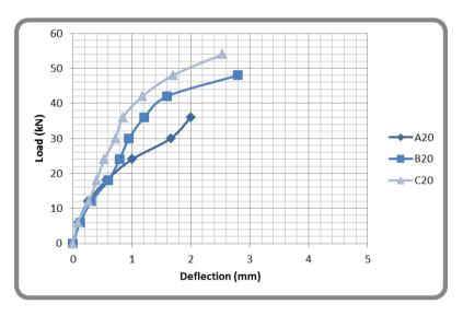
Fig. (8): Load –deflection curve for SCC T-section beam specimens without stirrups
