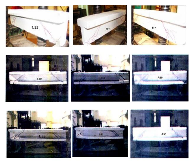
Fig (18): Crack patterns of the tested SCC beam specimens
