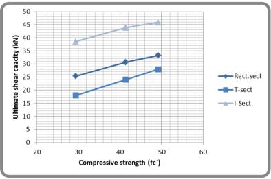
Fig. (12): Effect of compressive strength.  $(f_c')$  on the ultimate shear strength for SCC beam specimens without stirrups
