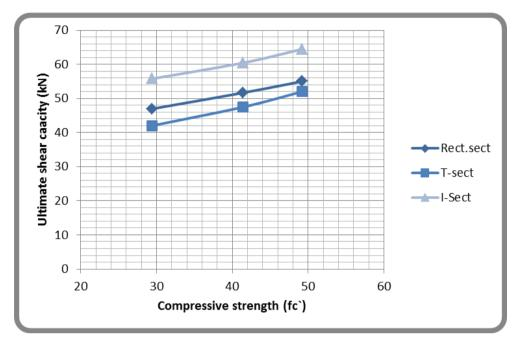
Fig. (13): Effect of compressive strength.  $(f_c^{'})$  on the ultimate shear strength for SCC beam specimens with stirrups
