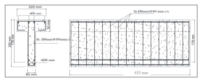
Fig. (2): Details of T-section (all dimensions in mm)
