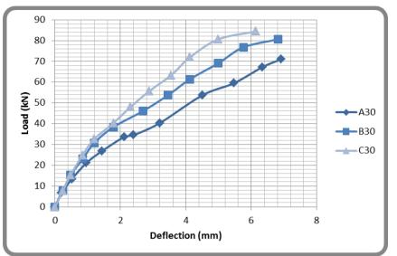
Fig. (10): Load –deflection curve for SCC I-section beam specimens without stirrups
