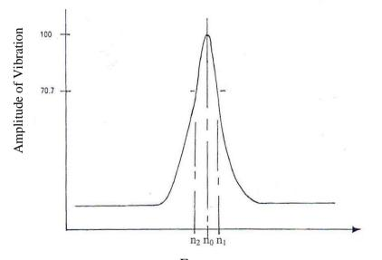
Frequency **Fig. (1):** Typical curve of amplitude of vibration with frequency
