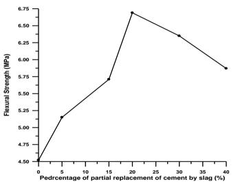
Fig. (5): The effect of slag as a partial replacement of cement on the flexural strength of concrete
