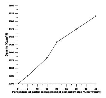
Fig. (3): The relationship between the density at (28 day) and the percentage of the replacement of cement by slag
