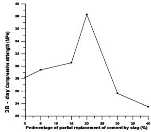
Fig. (4): The effect of slag as a partial replacement of cement on the compressive strength of concrete
