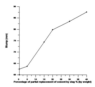
Fig. (2): The effect of slag as a partial replacement of cement on the workability of concrete
