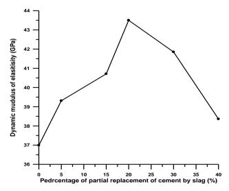
Fig. (6): Effect of partial replacement of slag on the modulus of elasticity of concrete
