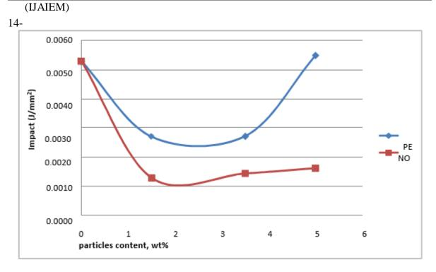
Fig. (1): impact strength of polyester vs. peach and novolac particles content
