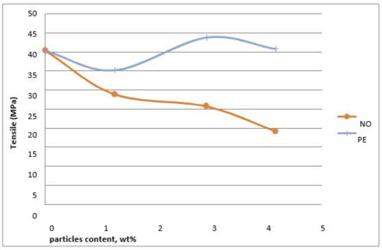
Fig. (3a): tensile strength vs. peach and novolac particles content
