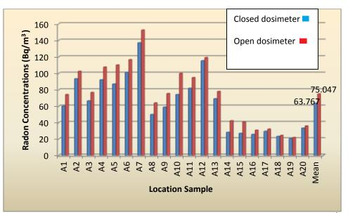
Figure3: A histogram illustrating the change in radon gas concentration (Bq/m<sup>3</sup>) in indoor dwelling samples for closed and open dosimeters in all regions studied.
