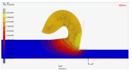
Fig. (2) Temperature distribution for case of 12° rack angle and 0.108 mm/rev feed
