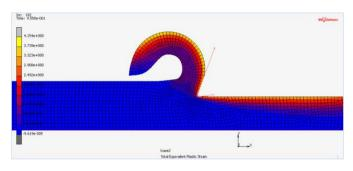
Fig. (3) Equivalent plastic strain case of 20° rack angle and 0.048 mm/rev feed
