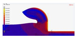
Fig. (1) Von Misses stress for case of  $0^{\circ}$  rack angle and 0.088 mm/rev feed
