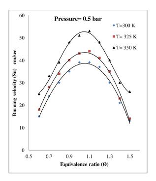
Fig. 5, temperature effect on laminar burning velocity for wide range of equivalence ratios at fixed P=0.5 bar
