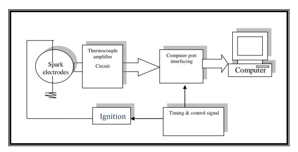
Fig (2) Block Diagram of Interfacing Circuit
