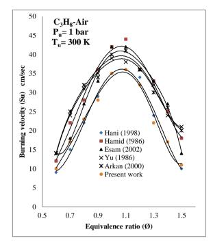
Fig. 3, comparison of present results with the published results of propane-air mixtures
