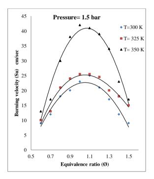
Fig. 6, temperature effect on laminar burning velocity for wide range of equivalence ratios at fixed P=1.5 bar
