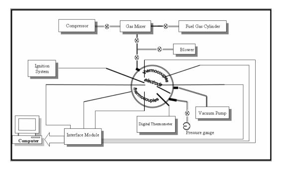
Fig. 1, Block diagram of experimental apparatus
