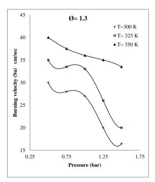
Fig. 6, pressure effect on laminar burning velocity for mixture equivalence ratio= 1.3 and variable temperatures
