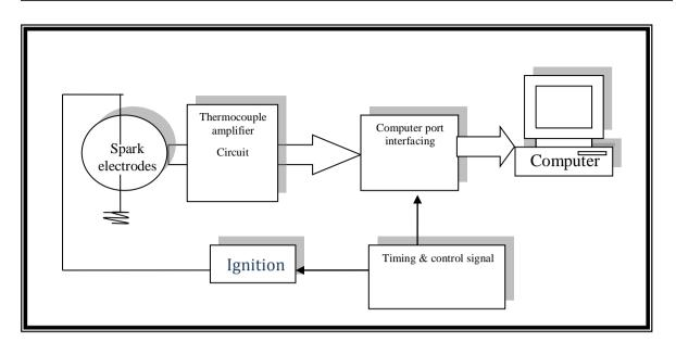
Fig (2) Block Diagram of Interfacing Circuit
