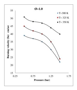
Fig. 5, pressure effect on laminar burning velocity for mixture equivalence ratio= 1.0 and variable temperatures
